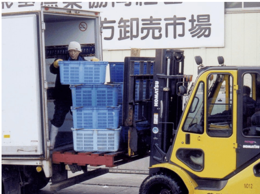
Figure 14: Hand-bombing cages from forklift into truck.
