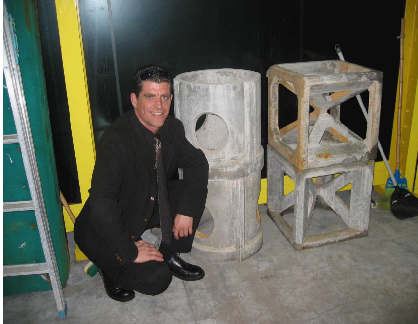
Figure 12: Concrete block design examples for artificial reefs (picture compliments of Dave McRae)
